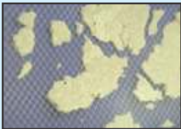
Scaling in RO Membrane
