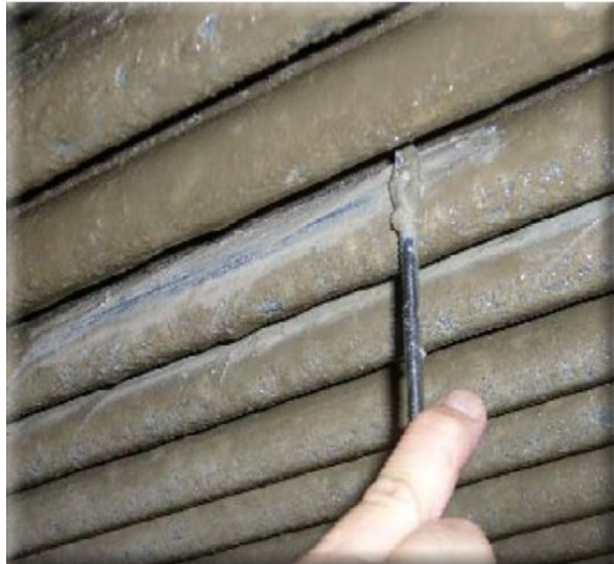
Scale thickness on tubes before installation was 2.00mm
