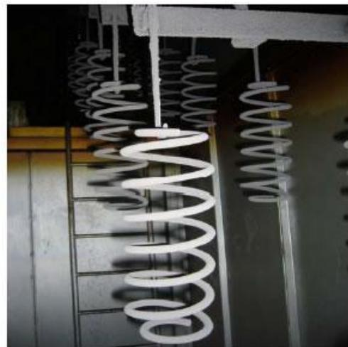
12. Coating quality weight on the coil spring should be having 7 – 15 gm/M2
