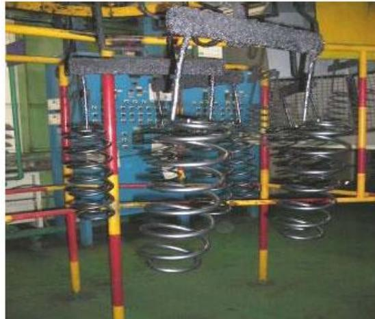
14. Coil Spring have been coating by Power Coating after
