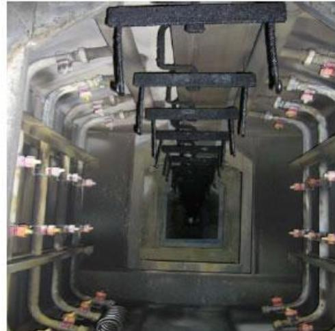
10. Zinc Phosphate , spray application are required the spray pressure at 1.5 – 1.8 Bar with to built up a crystal uniform coating on the spring substrate.
