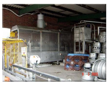
At Elgood's Brewery at Wisbech Cambridge the water is very hard with 330mg of Calcium and severe scaling was experienced particularly in the cask washer and also in the Angeleary Heater.
