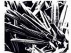
Treated calcium carbonate shown here in its colloidal crystal state
