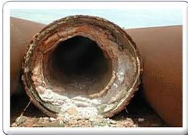
One area where scale will cause a problem is deposition inside the main feed pipes. Particularly hard water will see a steady build up of scale inside the pipe. This causes a reduction in water delivery, increasing the workload on the pumps. Furthermore scale can also contribute to corrosion of the pipe itself.
