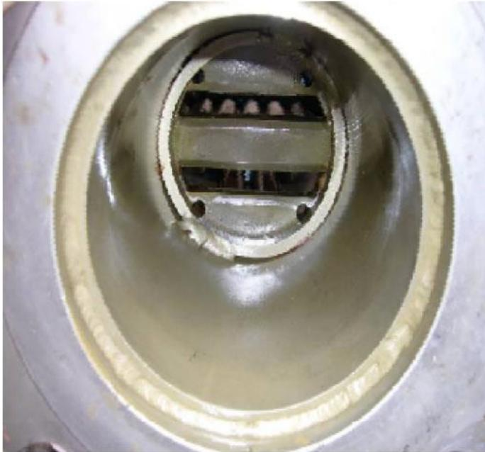
The MagCat was removed and inspected for fouling. There was no build up of any solids, just a coating of oil inside the unit.
