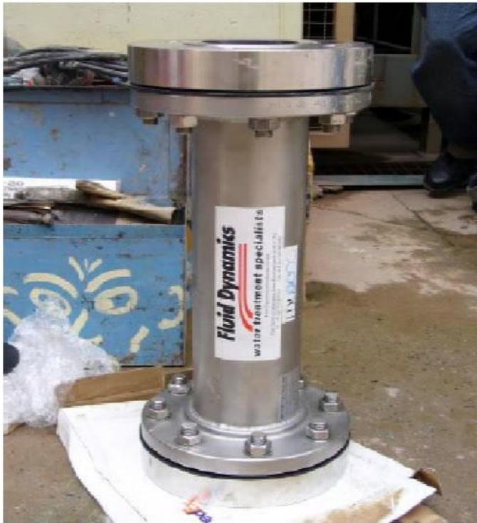
A proto type MagCat that combines Magstream and Colloid-A-Tron technology was installed due to the presence of oil in the system which could pose a problem for the Colloid-A-Tron.
