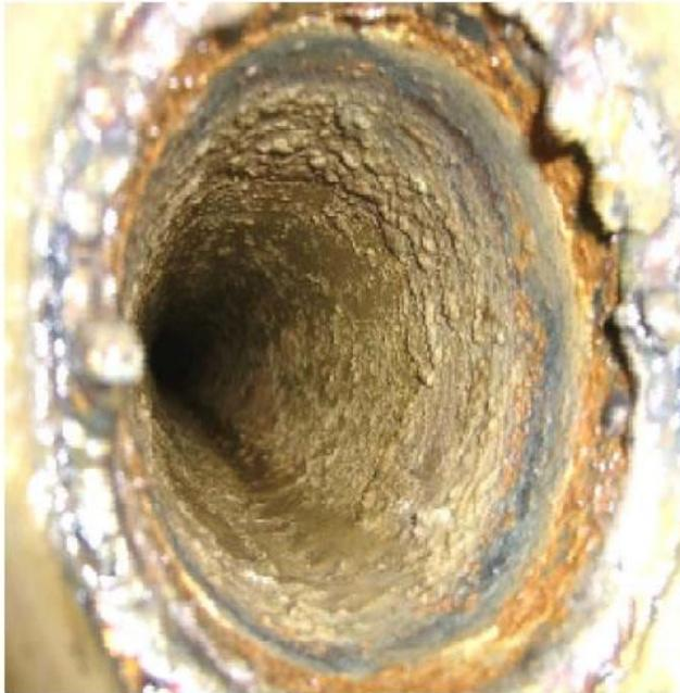
Once the MagCat was removed it was clear that the MagCat was having a considerable effect on the system. The scale thickness had decreased from 10mm to 3mm, a drop of 7mm.
