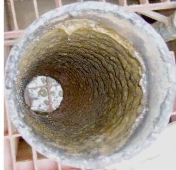
The thickness of scale inside the pipe was an average of 10mm decreasing the flow. The scale had also increased the weight of the pipe and, with much of it being installed on the ceiling, there were concerns that it could become unstable with the potential danger of it collapsing.
